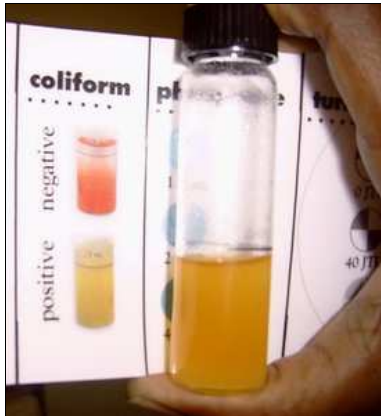
Test results show high levels of Coliform bacteria in Savannah Bay sea water...yuck!!!!
